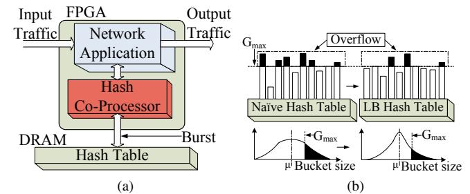
Fig. 1: (a) The proposed co-processor architecture. (b) The LB hash table reduces number of overflows compared to the naïve hash table and provides an even distribution of keys, where the bucket size (*i.e.*, number of keys in a bucket) distribution is denser around the average load,  $\mu$ .
