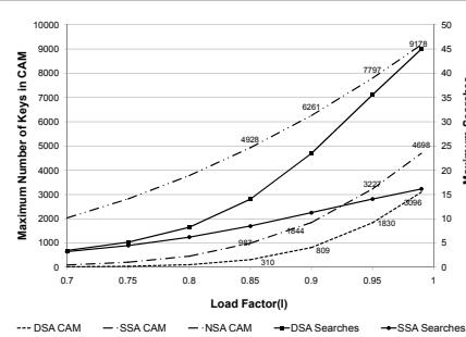
Fig. 5: Maximum number of keys in CAMs and maximum search time for different load factors.
