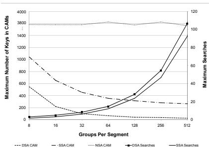
Fig. 4: Maximum number of keys in CAMs and maximum search time per insert operation.
